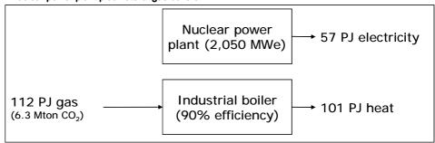
Reference situation with a CHP plant, and the new situation where the electricity is delivered by a nuclear power plant and the heat by a high-efficiency industrial boiler. Assumptions: CHP with an electric efficiency of 27% and a thermal efficiency of 50%. Nuclear power plant  $(2,050 \text{ MW}_e)$  running 7,684 hours per year. Industrial boiler efficiency: 90%.  $CO_2$  emissions natural gas: 56.1 kg  $CO_2/GJ$ .  $CO_2$  emissions coal: 97 kg  $CO_2/GJ$ .
