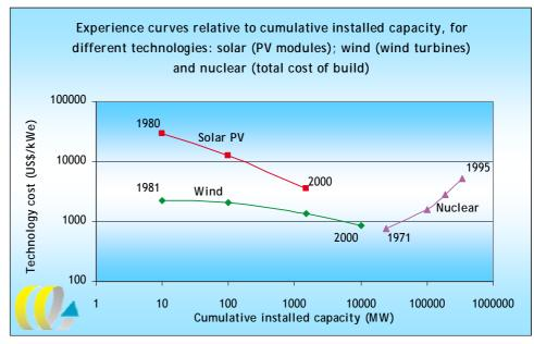
The figure indicates that the cost of PV-components and wind turbines has declined (although since 2000 the price of wind turbines has fluctuated), while the cost of nuclear has consistently risen (figure shows total cost of build).
